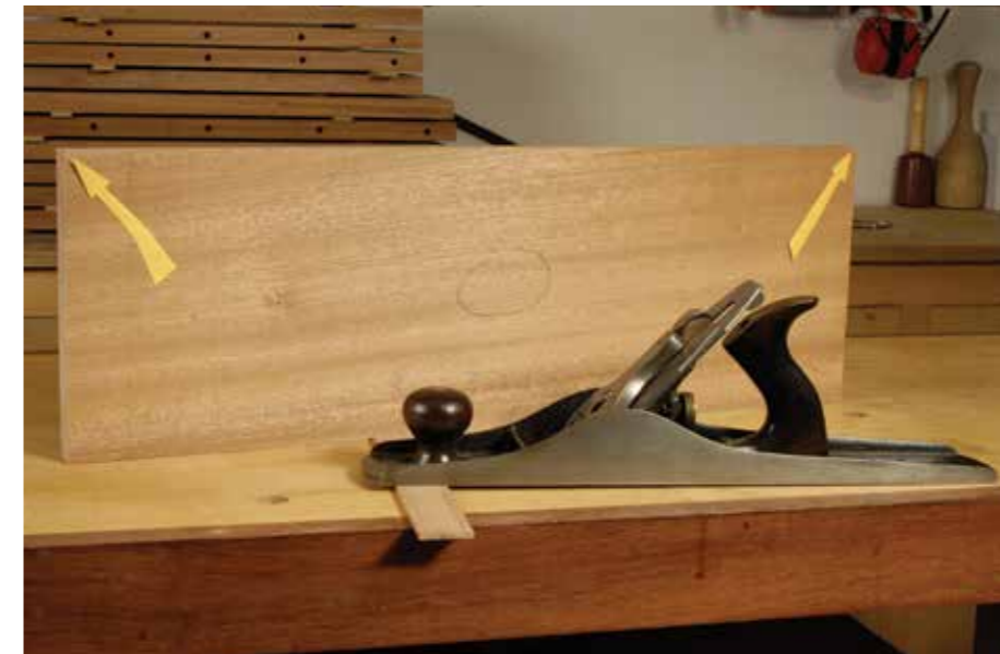
Starting and finishing with the blade off the timber, we are now moving back in the direction of convexity. Keep checking for squareness with the face side
