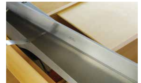
The correct way to inspect a plane sole, using feeler gauges and a reliable straightedge
