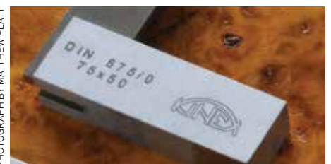
The DIN or BS mark on a measuring tool identifies the standard to which it was manufactured
