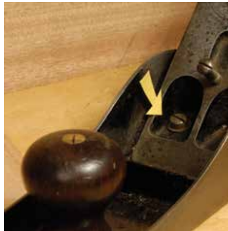
The sole of a bench plane can be distorted – or corrected – by a thou or so just by altering the tension on the knob, frog and handle screws. The big casting rib in front of the mouth ensures maximum sole stability at the most critical spot
