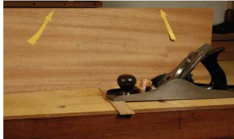
Taking a series of progressively longer stopped shavings, starting from the arrows, will generate concavity in the length of the edge
