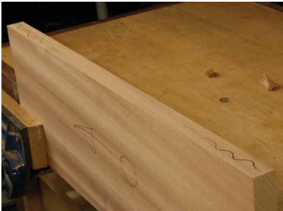
At this point the board is concave the plane will cease to cut, time to replace your pencil line and switch to through shavings
