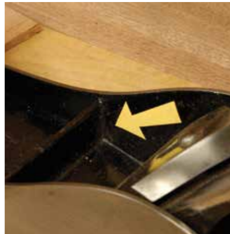
The sole of a bench plane can be distorted – or corrected – by a thou or so just by altering the tension on the knob, frog and handle screws. The big casting rib in front of the mouth ensures maximum sole stability at the most critical spot
