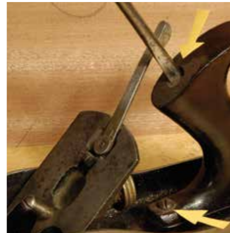
The sole of a bench plane can be distorted – or corrected – by a thou or so just by altering the tension on the knob, frog and handle screws. The big casting rib in front of the mouth ensures maximum sole stability at the most critical spot
